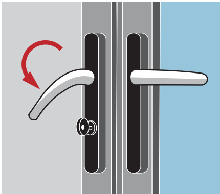
Fig 30. Push the handle down to retract the latch bolt and hook bolts. This allows the primary door to be opened.
